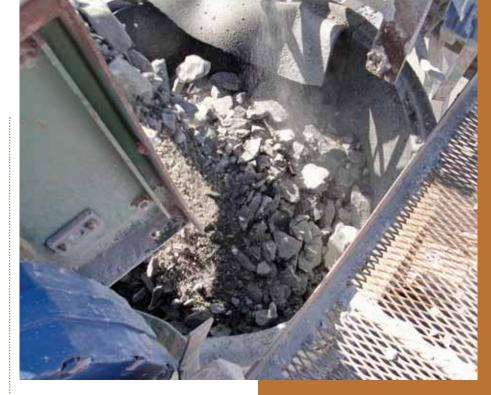
final screens, and crushing to the required top size earlier in the process. This will have the effect of freeing up capacity on the final screens and their feed conveyors by reducing the overall feed volume and increasing the available area for the remaining separations.
