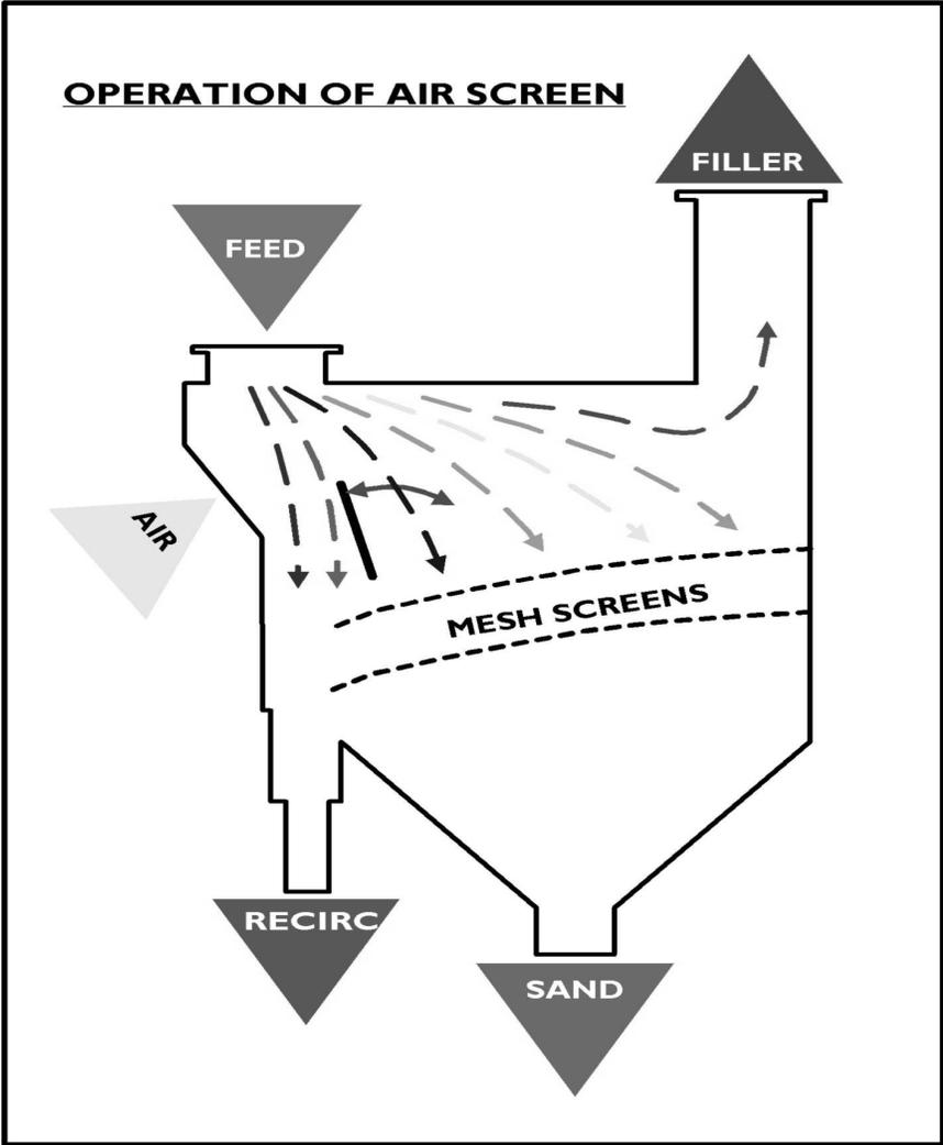
Fig. 4 Operation of air screen
