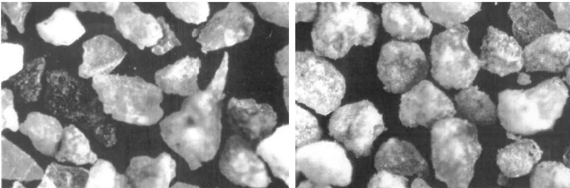
**Fig. 3** Comparison of 2.5mm-1.5mm grains before and after VSI crusher.
