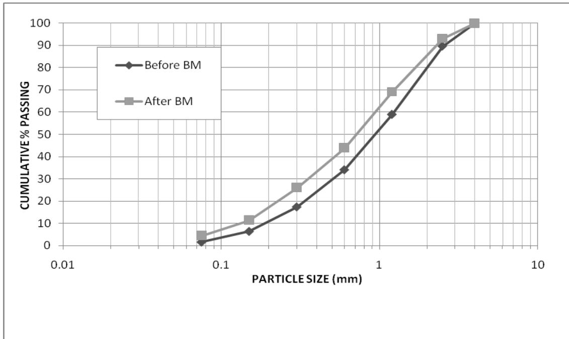
**Fig. 2** Example of change in size distribution due to Kemco VSI, running with 20% water content.
