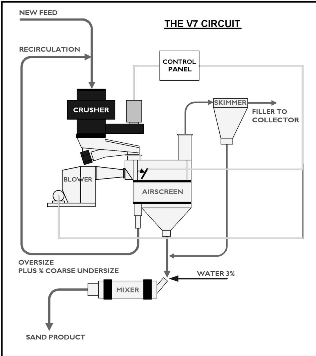
Fig. 5 V7 Circuit diagram
