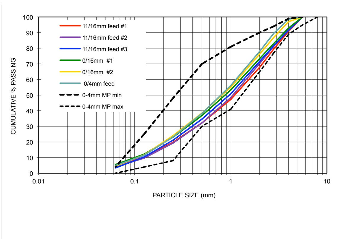
While it is tolerably easy to reduce the filler content to six or seven percent with feeds up to about 2% moisture, we have found that it needs to be less than 1% to achieve very low levels of filler. Granite material taken directly from a contract cone crusher on site was satisfactory providing that dust suppression with water sprays - never an effective method - was not used.
