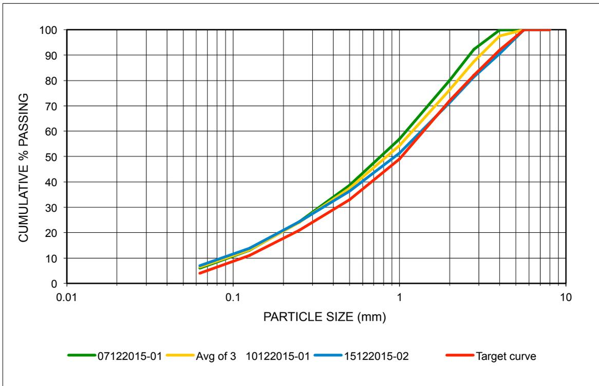
The graph above shows the effect of changing the aperture of the first screen cloth on the top deck from 4mm, through 5mm to 6mm, leaving the remainder of the deck at 4mm.
