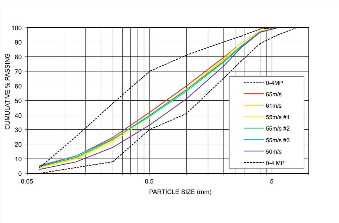
At the same time, there appears to be very little difference in the shape results whether the rotor speed is 50 or 65m/s, and longer term testing is needed to find the optimum.
