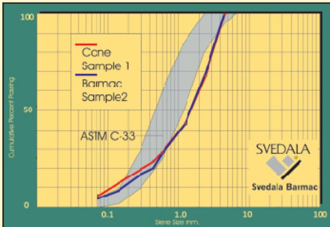
**Graph 3: The two gradations of minus 4.75 mm products. Note that the Barmac product is slightly coarser at the fine fraction (minus 1.0 mm) which will have a detrimental effect on voids and flow results due to the smaller volume of ultra fine material.**
