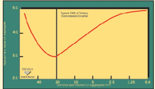
Graph 6: The closer the line gets to the axis on this graph represents the more equidimensional the particle shape.
