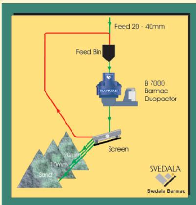
**Graphic 4: Tertiary crushing circuit for the production of high quality concrete sands and aggregates.**
