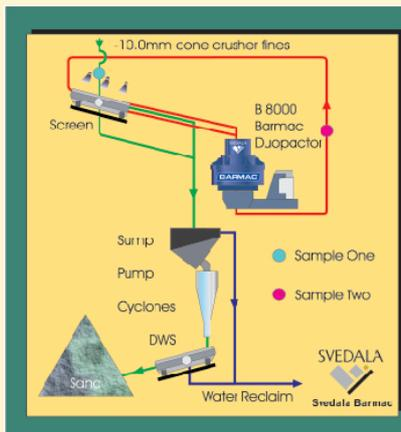
**Graphic 3: Crushing circuit for the re-processing of quarry fines. The feed to the Barmac Duopactor is minus 10 mm cone crusher product. The cone crusher product is screened at 3.0 mm and the remaining 3.0 mm - 10.0 mm is fed to the Barmac. The Barmac product is screened at 5.0 mm and the oversize re-circulated.**
