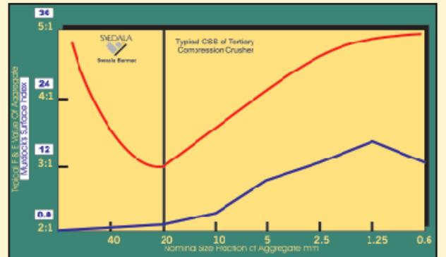
Graph 7: Note that the particle shape of an aggregate needs to be at the highest point on Murdock's surface index. Note that the requirement for good particle shape does not typically correspond with the setting at which a compression crusher produces its best particle shape.
