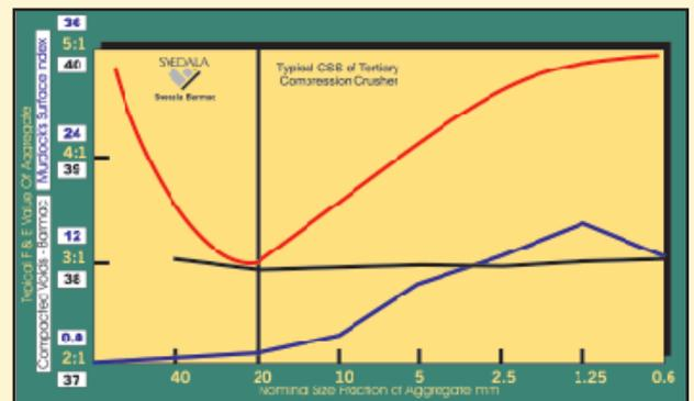
Graph 8: Note that the particle shape of the materials that have passed through the Barmac Duopactor remain relatively constant, especially at the size fraction that Murdock has established as being the most critical for concrete sands.
