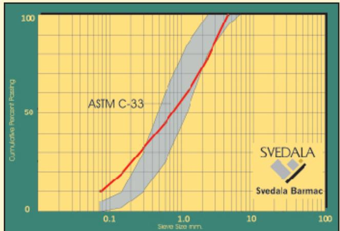
**Graph 5: Minus 4.75 mm gradation of the Barmac sand generated from the tertiary crushing circuit.**
