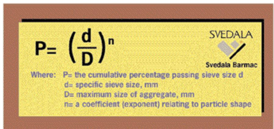
Graphic 1: Talbot's formula for calculating the theoretical gradation for minimum voids contents in sand.
