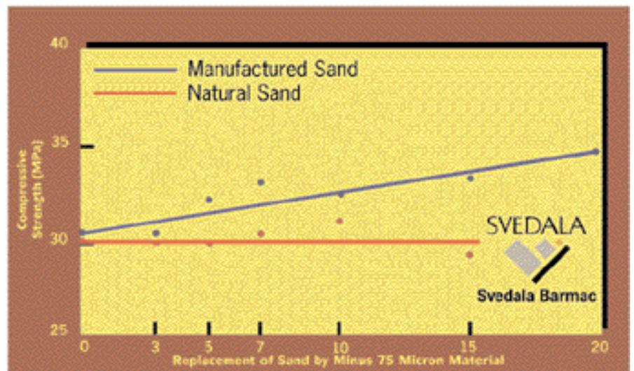
Graph 2: Source, Ahmed E Ahmed and Ahmed A. El-Kourid. - Properties of Concrete Incorporating Natural and Crushed Stone Very Fine Sand. ACI Materials Journal, Vol. 86, No 4, July 1989. pp 417 - 424.
